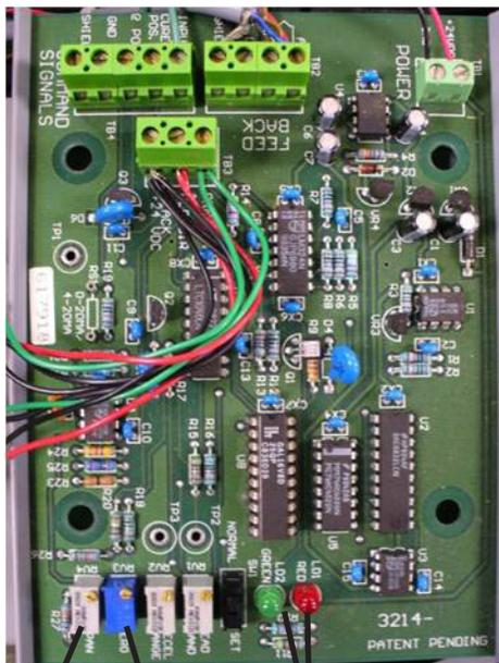
**Identify LEDs and Span and Zero adjustments.**
