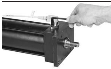
Bolt sensor to cylinder.
